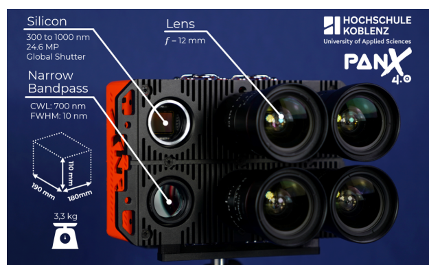
Figure 1. Newly developed 6-band VNIR multispectral multicamera system, PanX.4.
