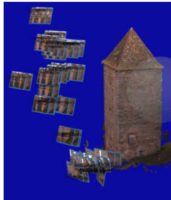
Figure 11. Postprocessed to a digital twin after stereoscopic inspection using the streamed image data
