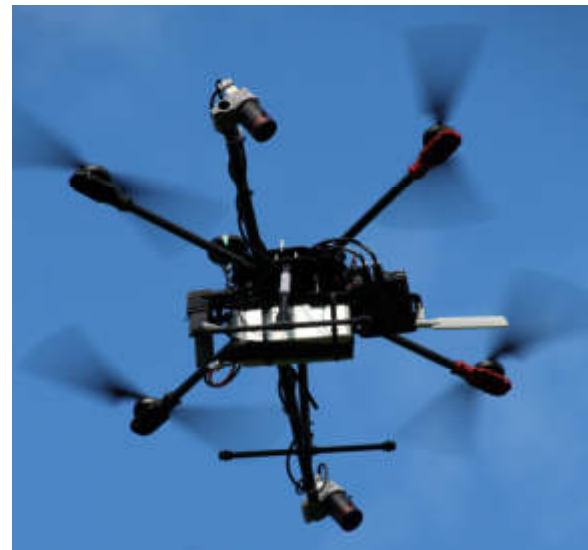
Figure 2. UAV as a MR generator equipped with the stereo cameras over a 1m base length
