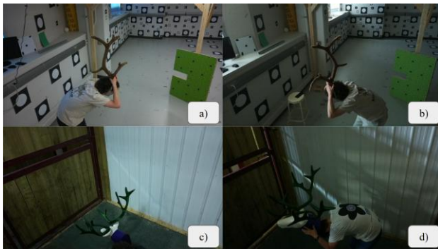
Figure 4: Frames from lighting conditions testing, (a) lab bright, (b) lab dark, (c) WRS bright, (d) WRS dark
