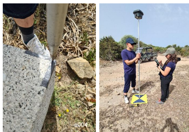
Figure 4. Examples of target materialized using Stonex S900A GNSS receiver.
