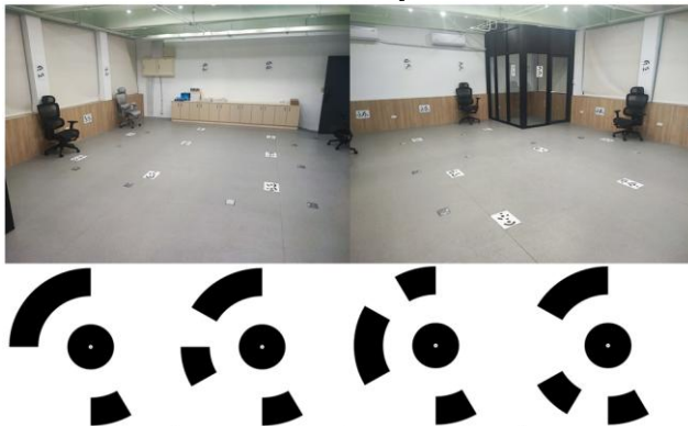
Figure 5. (a) Indoor calibration field (b) Control point pairs with known scale.
