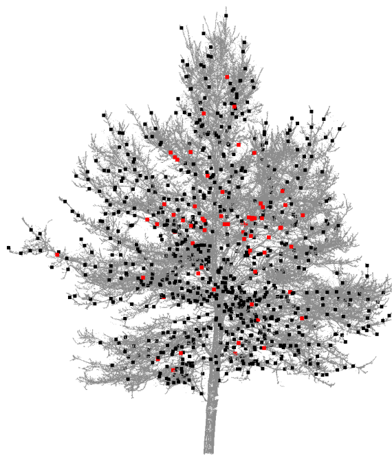
Figure 6. Point cloud of epoch E_0 showing 883 initial tracking points (black dots) and 48 selected tracking points (red dots) used for temporal resolution analysis.
