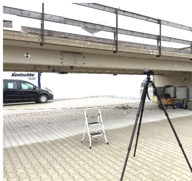
Figure 5. Measurement setup consisting of a consumer camera mounted on a stable tripod.
