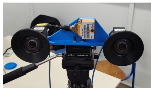
Figure 2. The custom-built stereo-inertial camera rig, showing the FLIR Blackfly S cameras and the STIM 300 IMU.
