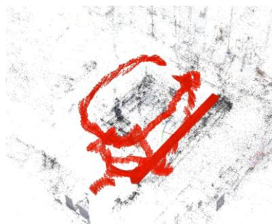
Figure 6. Visualization of the photogrammetric ground-truth trajectory (red) overlaid on the sparse 3D model of the linear guide environment generated by COLMAP.
