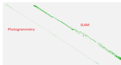
Figure 7. Visual comparison Experiment 1. Photogrammetry trajectory and ORB-SLAM 3 trajectory.
