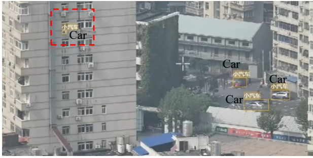
Figure 1. Example of a vehicle detection(YOLO v11) logic error in UAV imagery. The air-conditioning outdoor unit enclosed by the red dashed box in the image was incorrectly detected as a car due to its square shape.
