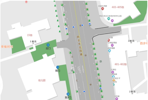
Figure 5. Schematic diagram of the experimental area. The gray area in the diagram represents high-precision road data collected through surveying and mapping, with lines indicating road centerlines, lane markings, road signs, etc. The white area represents building outline data, while the green area represents urban vegetation and green spaces.
