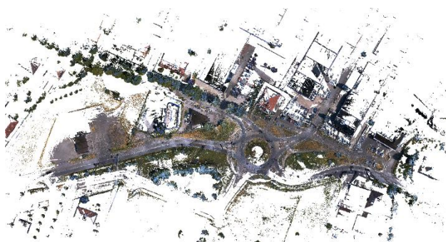
Figure 9. Top view of the LiDAR point cloud acquired through Riegl VZ-600i by the Laboratory of Geomatics.
