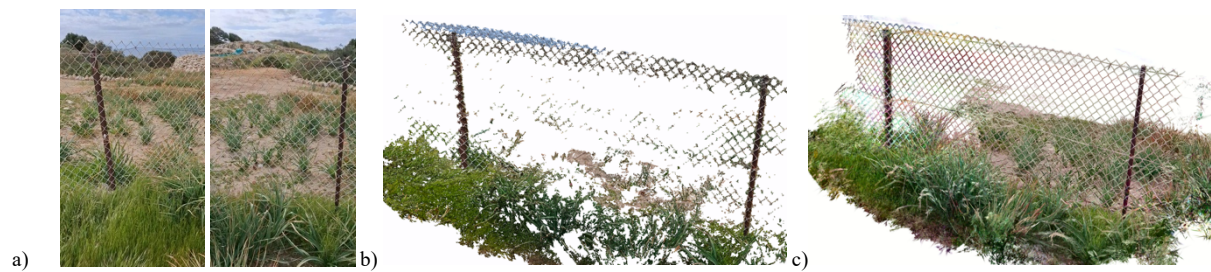
Figure 1. A thin metallic structure (a) reconstructed with a conventional photogrammetric MVS method (b) and GS (c).
