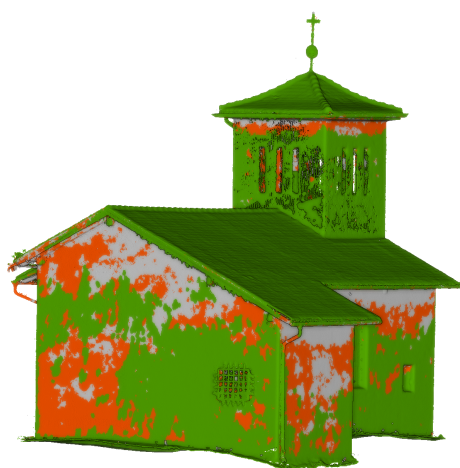
Figure 7. Detailed comparison of the completeness of the different methods. Green areas could be reconstructed by both methods, whereas red areas were only reconstructed by the NeRF point cloud. Grey areas could not be reconstructed successfully by either method.
