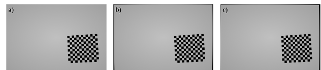
Figure 5. Qualitative comparison of distortion effects. (a) Undistorted reference image. (b) distortion using ground-truth parameters. (c) distortion using predicted parameters. The predicted distortion produces a similar global deformation with slight boundary shifts.
