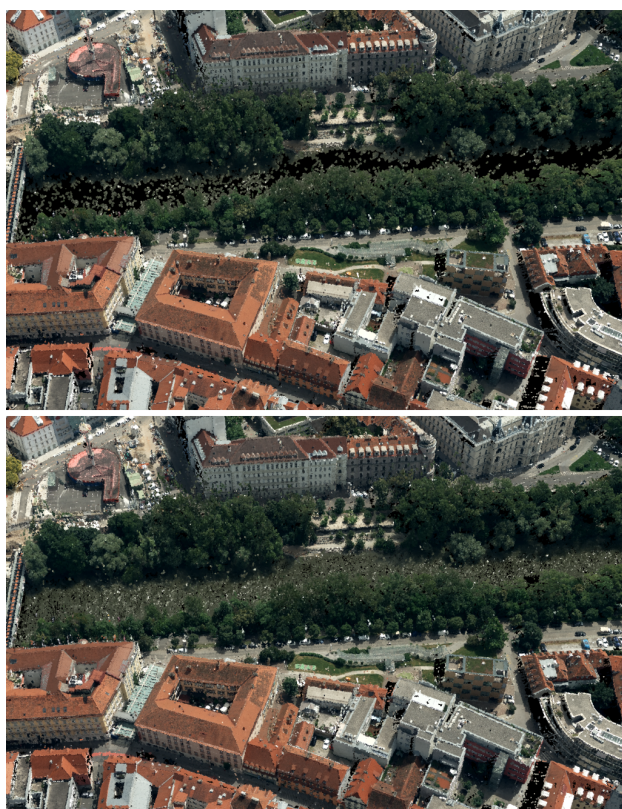
Figure 3. One-view point cloud comparison: The top image shows the initial photogrammetry result, while the bottom image illustrates the improved completeness and consistency after registration and LiDAR integration.
