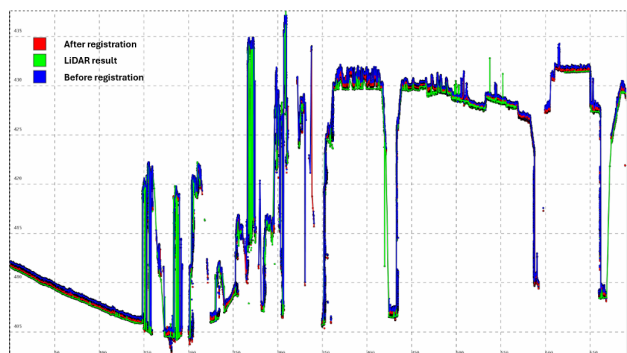
Figure 5. Vertical profile analysis demonstrating that the registered elevation (Red) aligns closely with the LiDAR reference (Green), significantly reducing the initial geometric drift (Blue).
