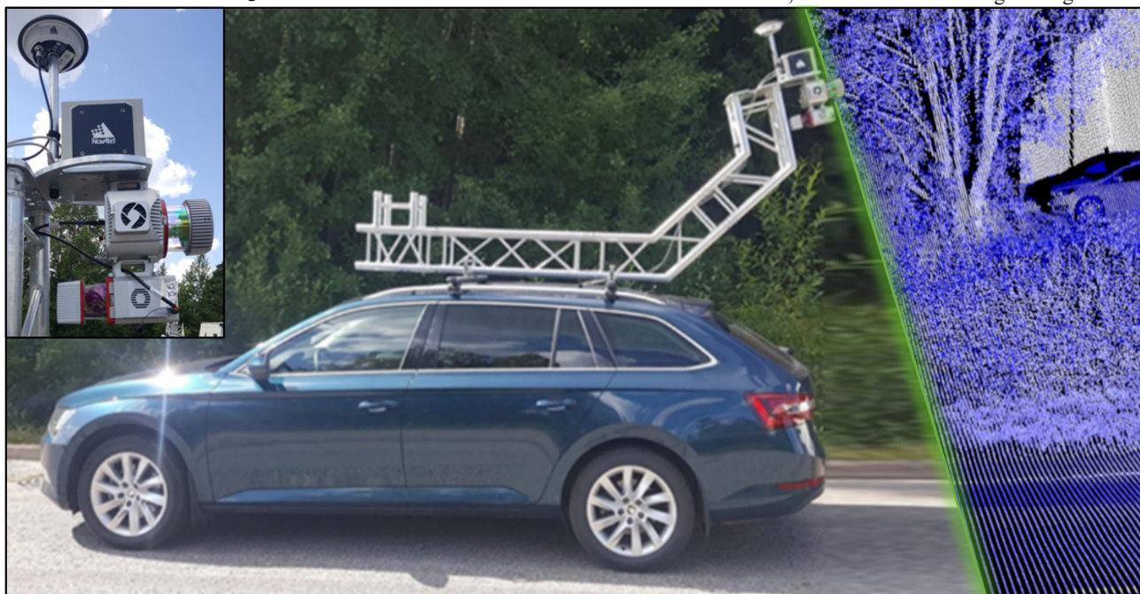
Figure 1. FGI Roamer-R4DW mobile mapping system used in this study. The figure shows the sensor configuration on the survey vehicle and illustrates the 360° scanning geometry and resulting point cloud coverage of the road environment (adapted from El Issaoui et al., 2026).
