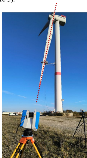
Figure 5. Measurement setup for the field experiment showing the TLS and rotor blade orientation.
