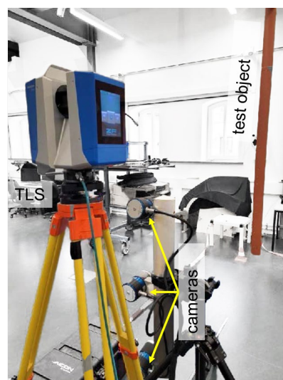
Figure 4. Laboratory experiment setup with TLS and photogrammetric reference markers (adapted from Harms, 2024).
