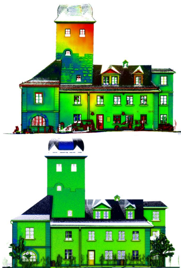
Figure 7. Side-by-side comparison of real (top) and simulated (bottom) point clouds.
