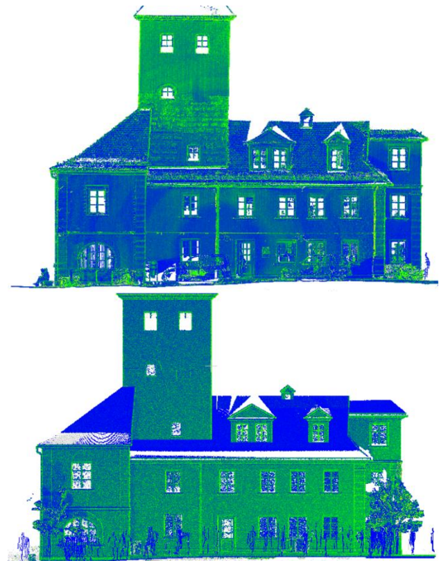
Figure 10. Roughness visualization of the real (top) and simulated (bottom) point clouds.
