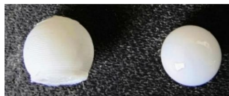
Figure 2. The tested marker models – 3D printed (left) and ceramic (right). Minor irregularities, which vary from marker to marker, can be observed in the 3D-printed model.
