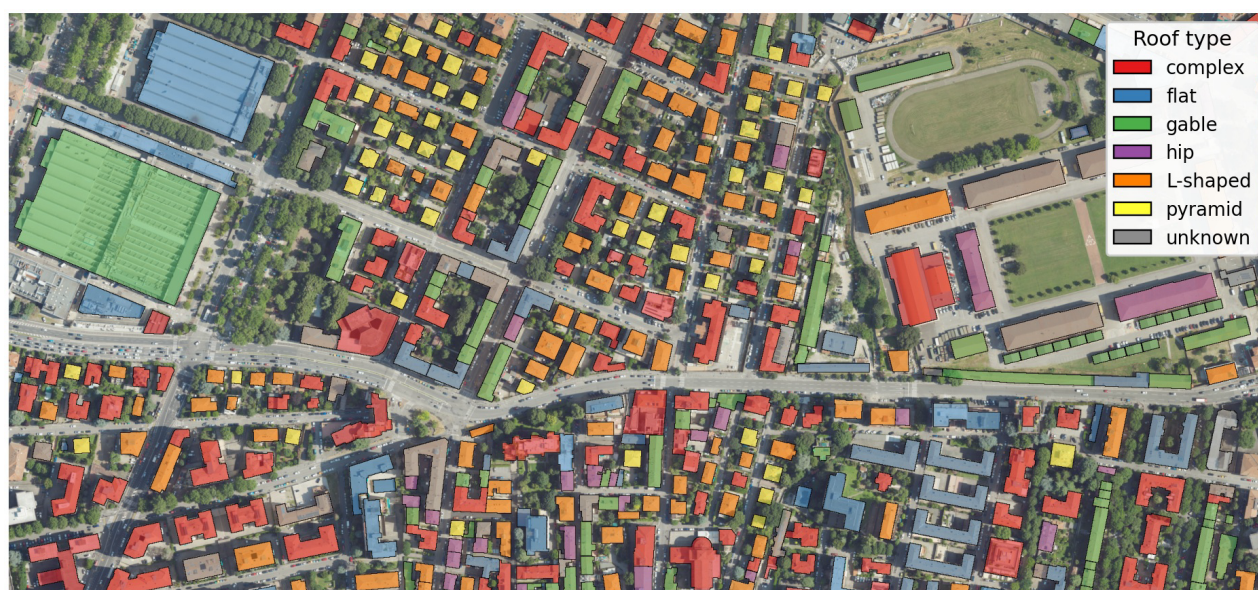
Figure 4. Roof type classification results for the Bologna reconstruction tile. Building footprints are coloured according to the predicted roof class, while uncertain cases are preserved as unknown for downstream fallback reconstruction.
