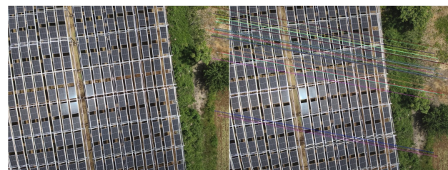
Figure 4. An image pair dominated by repeated patterns for matching. By using SIFT-StereoGlue method, only 42 robust matches were found.
