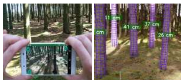
Figure 1. Example of high-resolution 3D reconstruction of the lower part of tree stems from terrestrial photogrammetry. Purple wireframe cylinders represent automated stem detection, with the estimated diameter at breast height for each detected stem.
