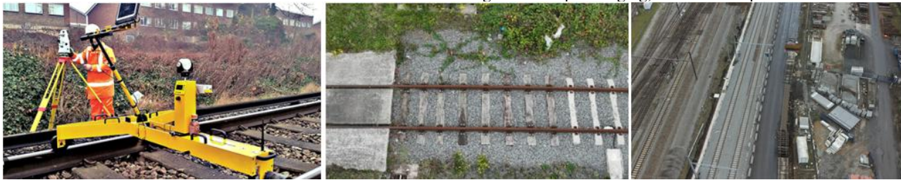
Figure 2: (left) Conventional GEDO survey trolley system, (middle) unconstrained UAV flight image ( A=5 m, GSD=2 mm) and (right) constrained conventional flight image ( A=30 m, GSD=11 mm).
