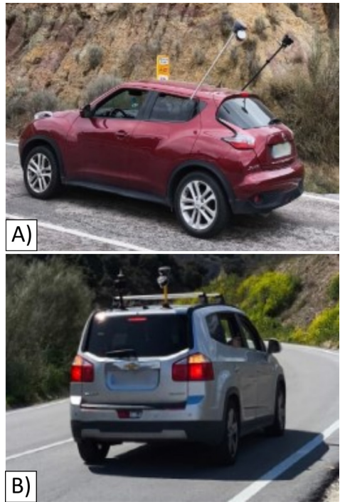
Figure 5. MMS mounting configurations: a) 2-meter pole mount; b) suction-cup mount.
