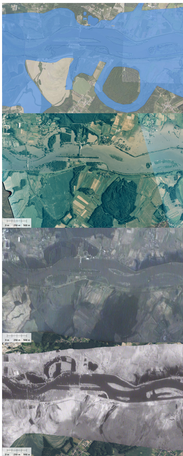
Figure 8. Visual comparison of 1997 Central European Flood range near Brzeg Dolny for different datasets. From top: Polish Hydroportal, aerial photos, RGB VHS orthomosaic (flight 2, increased brightness), NIR VHS orthomosaic (flight 2) with the 2025 orthophotomap in the background.
