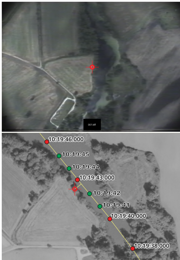
Figure 4. Example of timestamp and position determination for the first and last image in the sequence. The top view shows an image with a marked center, the bottom view shows the image center in the archival orthophotomap projected on the trajectory (yellow line) with marked time stamps (red dots show trajectory points, green dots are 1 s interpolated timestamps).
