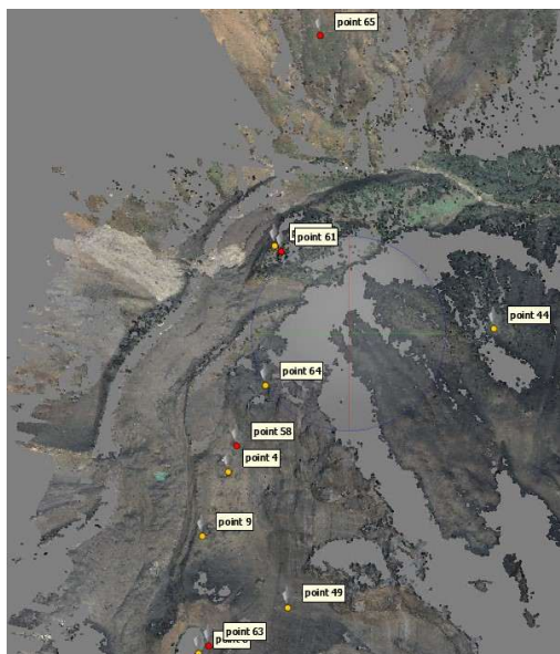
Figure 6. GCPs (in orange) and CPs (in red), 2023 model
