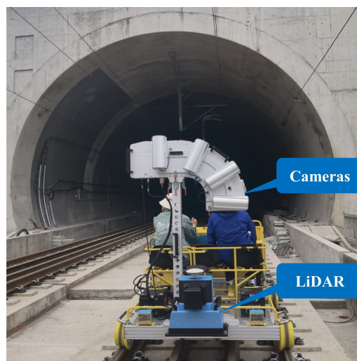
Figure 1. Harsh tunnel environment (low light, low texture, dynamic flash) and the integrated LiDAR–camera mapping system mounted on a rail-based platform.
