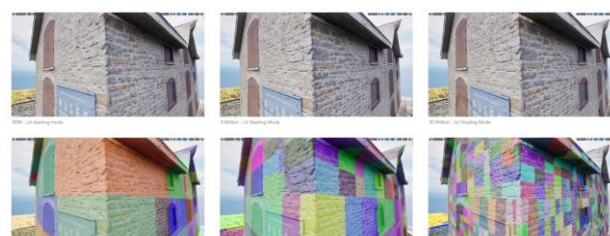
Figure 4. 3D Tiles output from the Mesh2Tile pipeline loaded in Unreal Engine 5 via Cesium for Unreal. Top row: lit shading mode at 900K (left), 9 million (centre), and 90 million (right) triangles. Bottom row: Cesium colorized tile debug mode at the same three scales, where each colour represents an individual tile.
