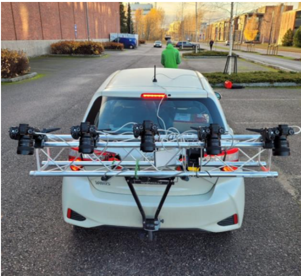
Figure 3. Mobile multi-camera system for photogrammetric road surface 3D measurements.
