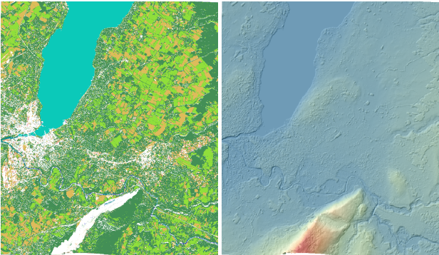
Border interpolation on Geneva (Switzerland) DSM (lake) Pléiades © CNES 2017, Distribution CNES PWH
