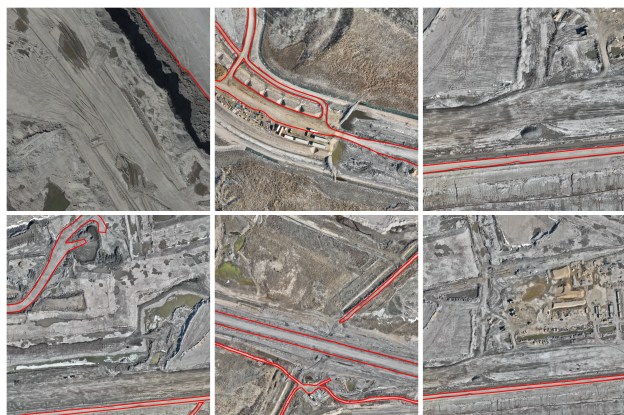
Figure 1- Aerial imagery samples of open-pit mine haul roads with extracted boundaries shown in red.
