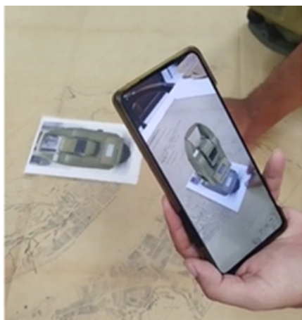
Figure 6. Augmented reality visualization of the optimized Wild T2 theodolite model using Unity and Vuforia
