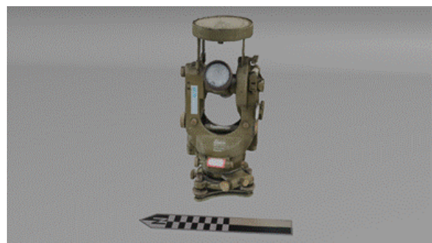
Figure 5. Optimized 3D model of the Wild T2 theodolite after mesh refinement and polygon reduction performed in Blender.
