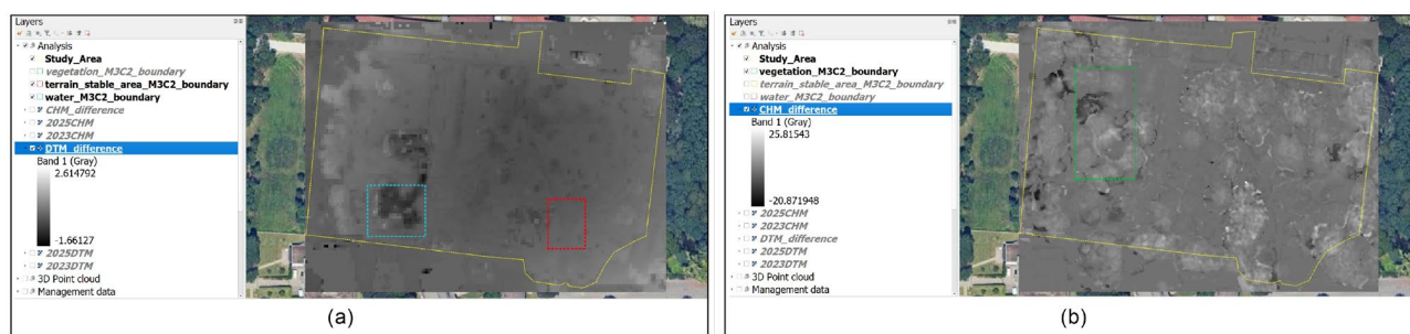
Figure 6. Feature-level interpretation of detected changes using GIS-based analysis: DTM difference (a) and CHM difference (b).
