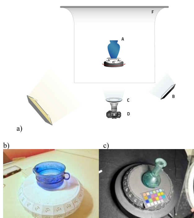
Figure 1. Rotating table setup with coded targets, a colour checker and white (left) or black (centre) background to support automated orientation processes.
