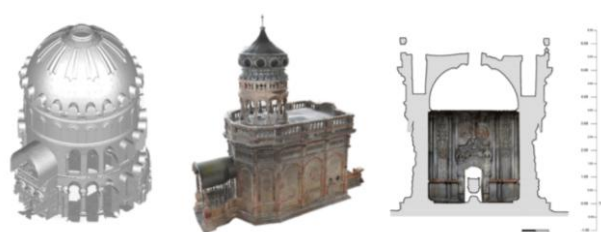
Figure 1. The results of the geometric documentation: point cloud, 3D textured model, orthoimage (left to right).
