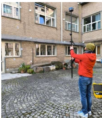
Figure 5. Example of data acquisition with the Stonex S999 for the GNSS-Ph approach
