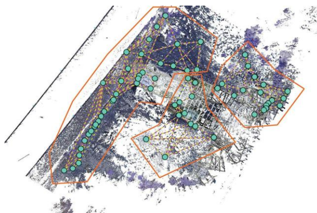
Figure 3. Laser scanning - three cloud-to-cloud registration bundles
