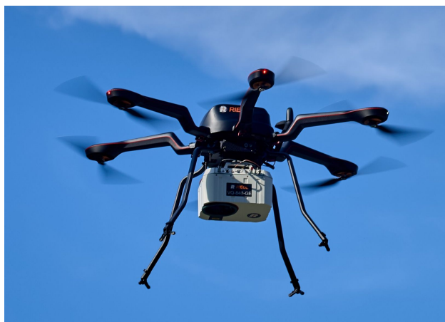
Figure 2. RIEGL VQ-840-GE airborne bathymetric laser scanner mounted on a UAS.
