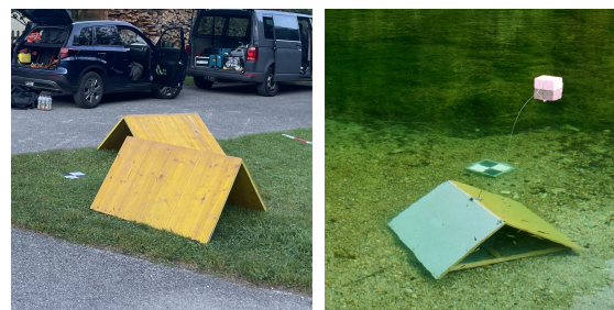
Figure 3. Planar reference geometry above (left) and below (right) the water surface.
