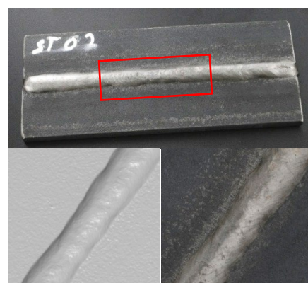
Figure 3. Top: test object, region of interest (ROI) is marked red. Bottom left: perspective view of the reference pointcloud in the ROI without texture. Bottom right: as left with texture.
