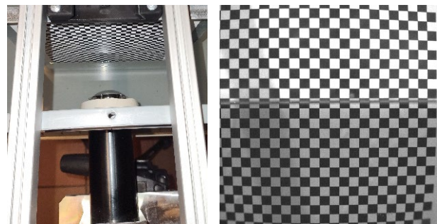
Figure 2. Left: top view of the camera tube penetrating the water basin. The camera is on the water-surface-level observing a chessboard target through the hemispheric interface. Right: camera image of the chessboard half in water half in air.
