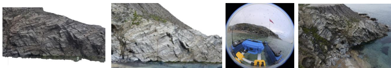
Figure 6. Side-by-side comparison between Insta360-based and UAV-based photogrammetric results. From left to right: (a) detail of the reconstruction derived from Insta360 images, (b) detail of the reconstruction derived from UAV images, (c) Insta360 input image, and (d) UAV input image.
