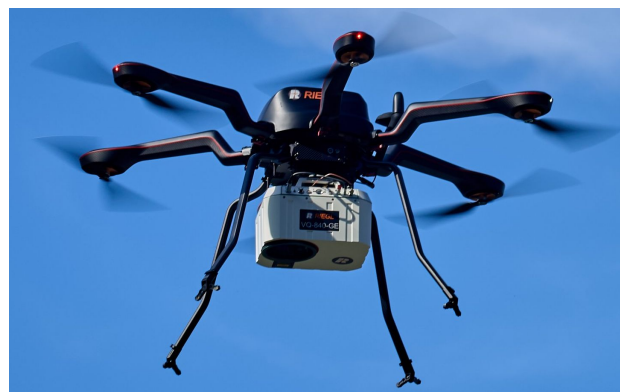
Figure 3. RIEGL VQ-840-GE topo-bathymetric laser scanner mounted on an Acecore Noa quadcopter UAV during data acquisition at Almsee in August 2025
