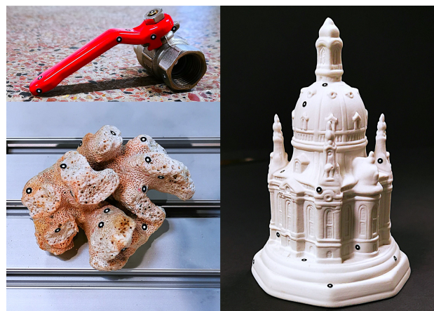
Figure 1. Test objects used for photogrammetric reconstruction: coral stone, church replica, and ball valve
