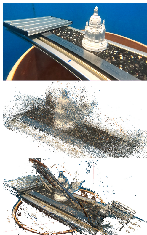
Figure 5. Example of a failed alignment: Object (top), resulting dense point cloud (center) and derived 3D model (bottom)
