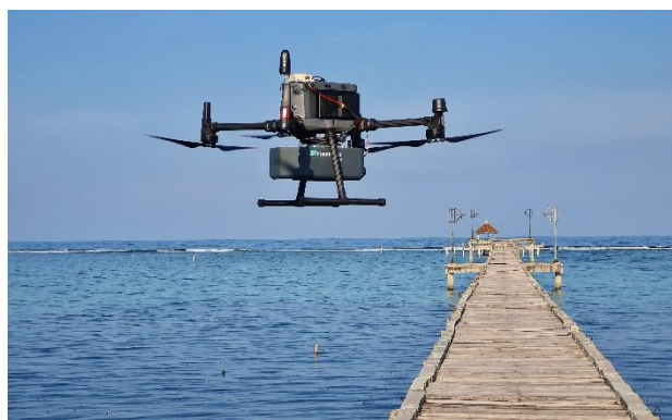
Figure 3: ABS (Fraunhofer IPM) mounted on a UAV
