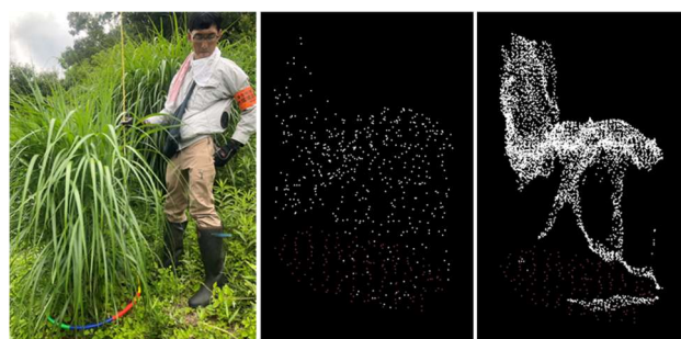
Figure 8. Ground vegetation survey plots (left), UAV LiDAR point cloud (middle) and UAV SfM point cloud (right). UAV LiDAR penetrates grass species more effectively, while UAV SfM provides higher-density surface data.
