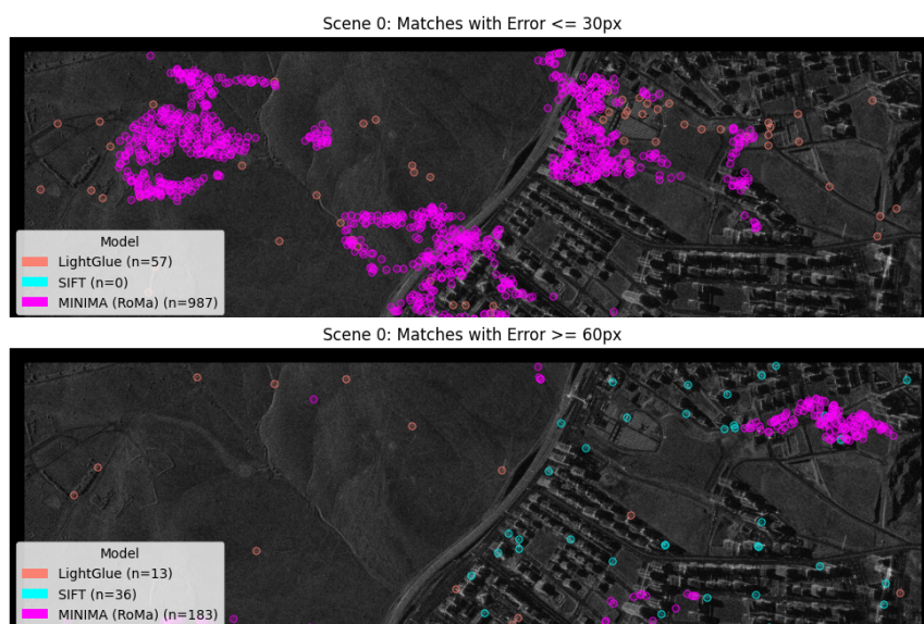
Figure 8. Distribution of positive and negative matches per matcher in one exemplary scene.
