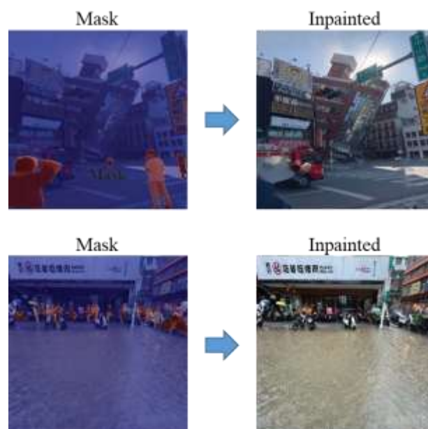
Figure 5. Example results of object masking and image inpainting. Dynamic objects such as vehicles and pedestrians are detected using Mask R-CNN (left) and removed through image inpainting to restore the background scene (right), improving image consistency for subsequent geolocation matching.
