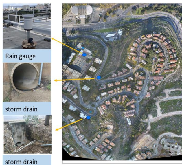
Figure 2. Monitoring infrastructure and measurement locations in the study area: the aerial orthophoto shows the locations of the rainfall gauge (installed at Romema kindergarten school), the upper drainage outlet (Tzolelet Dakar Street), and the lower drainage outlet (HaPerachim Street), marked with blue dots. Photographs on the left show the rain gauge and drainage conduits at the respective locations
