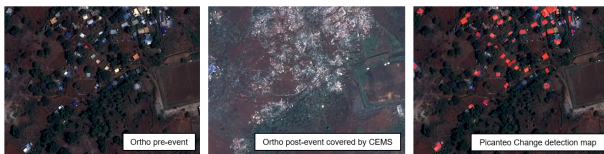
Figure 6. Missing destroyed building by Copernicus Emergency Management Services. Left: Pre-event orthoimage; Middle: Post-event orthoimage; Right: PICANTEO bi-temporal 2D detection pipeline output. Pléiades ©CNES 2024/2025, Distribution CNES PWH.
