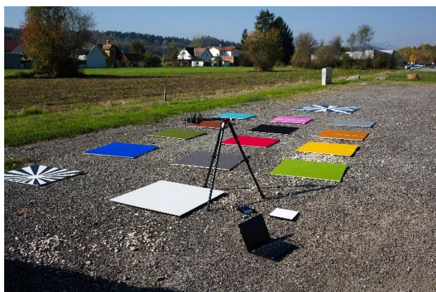
Figure 1. Color and reflectance target measurements during an aerial flight mission
