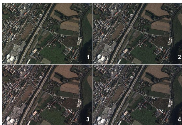
Figure 6. Gleisdorf image, original Level02 image (1), reflectance image from Level02 image (1), radiance image (3), reflectance image (Level03) from estimated Scale Factor computation (4)
