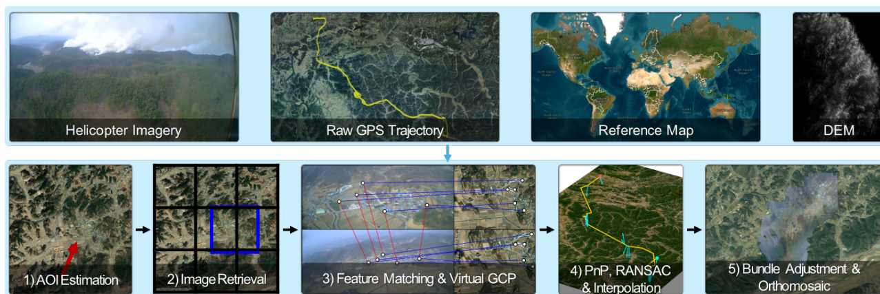
Figure 1. Overview of the proposed georeferencing pipeline from oblique helicopter imagery to orthomosaic output. Basemap: Esri World Imagery ©2026 Esri.
