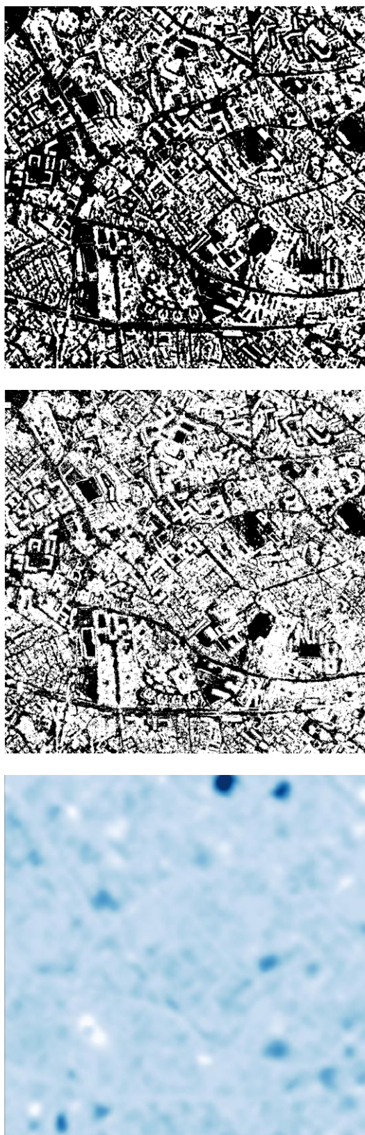
Figure 5: Comparison of ground masks derived using PDAL/CSF (top) and SAGA (middle), and their impact on the DTM. Bottom: elevation difference ( DTM_{SAGA} - DTM_{PDAL} ), ranging from -1 m (light blue) to +3 m (dark blue). The figure illustrates the different behaviours of the two filters and their influence on terrain reconstruction.
